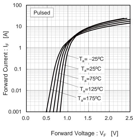
Fig.2  $V_F$  -  $I_F$  Characteristics
