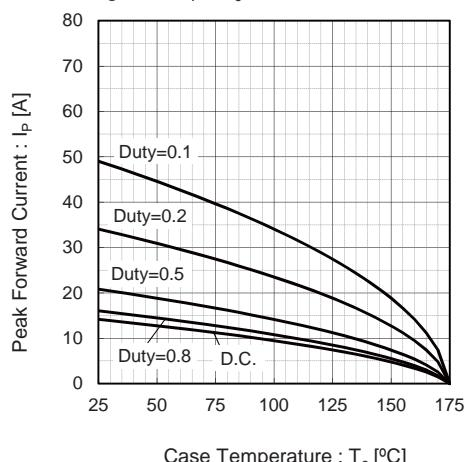
Fig.8<sup>\*4</sup> Typical peak forward current derating curve  $I_P$  -  $T_c$  (Not guaranteed)
